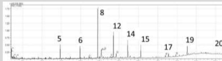
Fig. 5 Chromatogram of black substance obtained from Py-GC/MS with TMAH derivatization, pyrolysed at 550degC. Peak 5: Octanoic acid methyl ester (C8), Peak 6: Decanoic acid methyl ester (C10), Peak 8: Dodecanoic acid, methyl ester (C12), Peak 12: Tetradecanoic acid, methyl ester (C14), Peak 14: Hexadecanoic acid, methyl ester (C16), Peak 15: Octadecanoic acid methyl ester (C18), Peak 17: Lup-20(29)-en-3-one, Peak 19: Hexakisnor-dammaran-3,20-dione, Peak 20: Ursolic acid methyl ester
